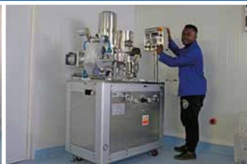
Tea bag making machine at ARC-VOPI, Roodeplaai
